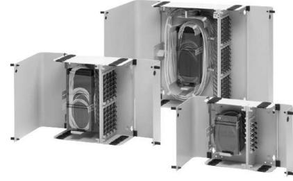
ADC's FL1000 customer premises fiber termination products include a variety of one and two door wall mount panels. These products are designed specifically to act as part of the fiber distribution system as the demarcation point for the service provider at the customers location.
